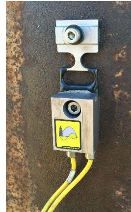
Combined sensors to be used on both steel and concrete piles, easy to mount with two bolts each only
