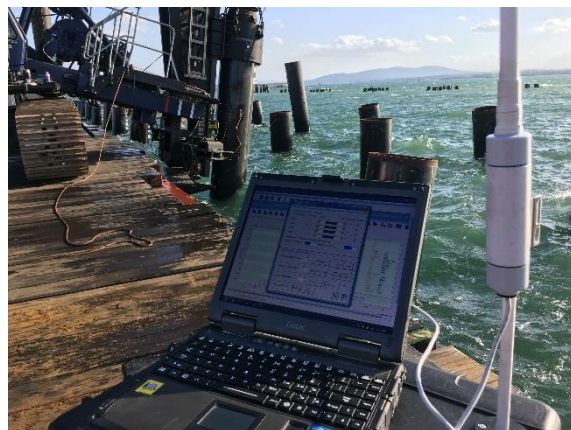
Monitoring during driving with the wireless monitoring equipment of Allnamics
