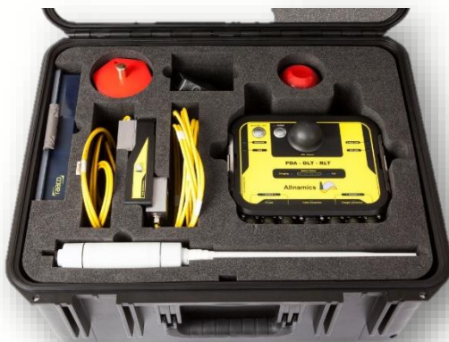
Complete set of PDA equipment and tools in transport case (29 cm x 45 cm x 55 cm, 15 kg)
