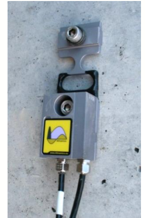
Combined sensors to be used on both steel and concrete piles, easy to mount with two bolts each only
