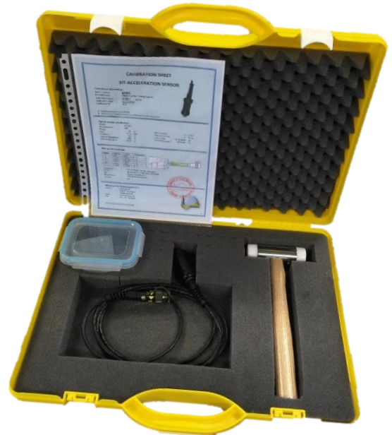
Complete set of SIT equipment and tools in transport case
