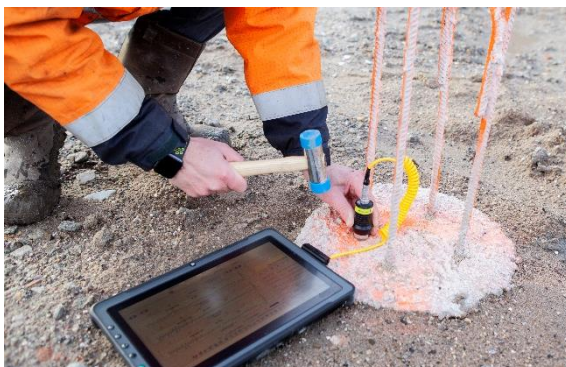
Sonic Integrity Testing to determine the conditions of foundation piles
