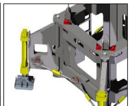
Bottom frame with hydraulically extendable legs.
